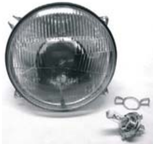
Fig. 4. Lamp 0215.8.10.8.0 produced by Zelmot with a H4 light bulb
