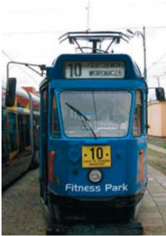
Fig. 1. Tram 13N with a single reflector 0215.8.10.8.0 produced by Zelmot (with a H4 light bulb)
