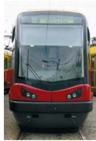
Fig. 3. Tram 120N with two low beam light projectors 1BL 008 193-01 (with a H7 light bulb) and two main light reflectors 1KO 008 191-02 (with a H7 Hella light bulb)
