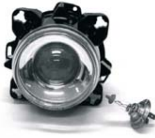
Fig. 10. Low beam light projector IBL 008 193-01 produced by Hella with a H7 light bulb
