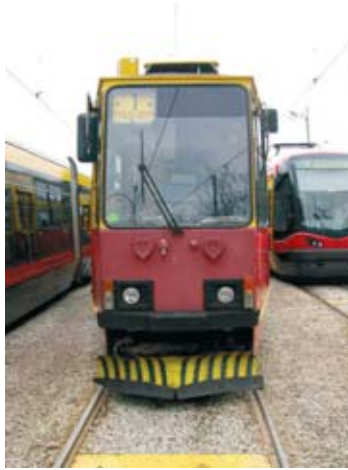
Fig. 2. Tram 105N with two reflectors 0245.2008.1 produced by Zelmot (with a R2light bulb)
