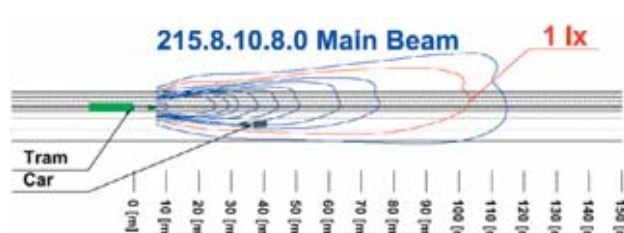
Fig. 15. Distribution of luminous flux density of reflector of lamp 0215.8.10.8.0 (H4), main light on road surface
